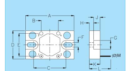
Best results can be reached by using a thermal transfer compound with a heat conductivity of better than 1W/mK.The flatness of the cooling plate must be better than 0.05mm overall. The roughness of the surface should not exceed 6.4µm.
