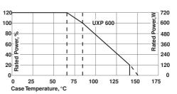
Derating (thermal resist.) UXP 600: 8.33W/°K (0.12°K/W) Power Rating: 600W at 85 °C bottom case temp.\*
