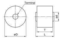
Molded with epoxide resin; alumina filler.
